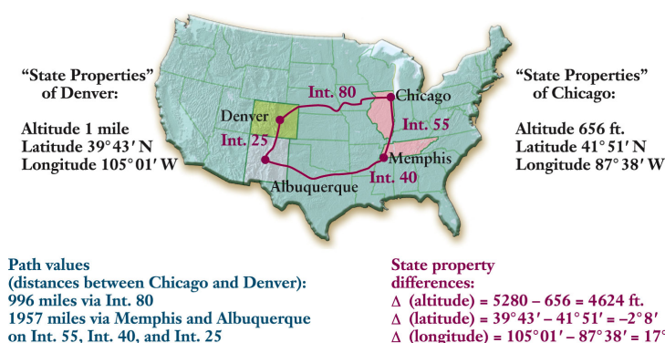
Fig. 12.3. Differences in state properties are independent of the path followed.
